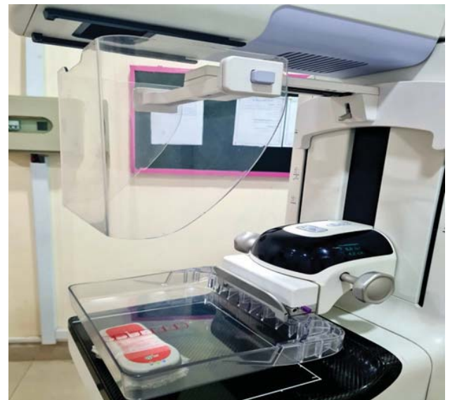
Figure 1: The X-ray Output ( X_{ref,4.5} ) Measurement Set-up
