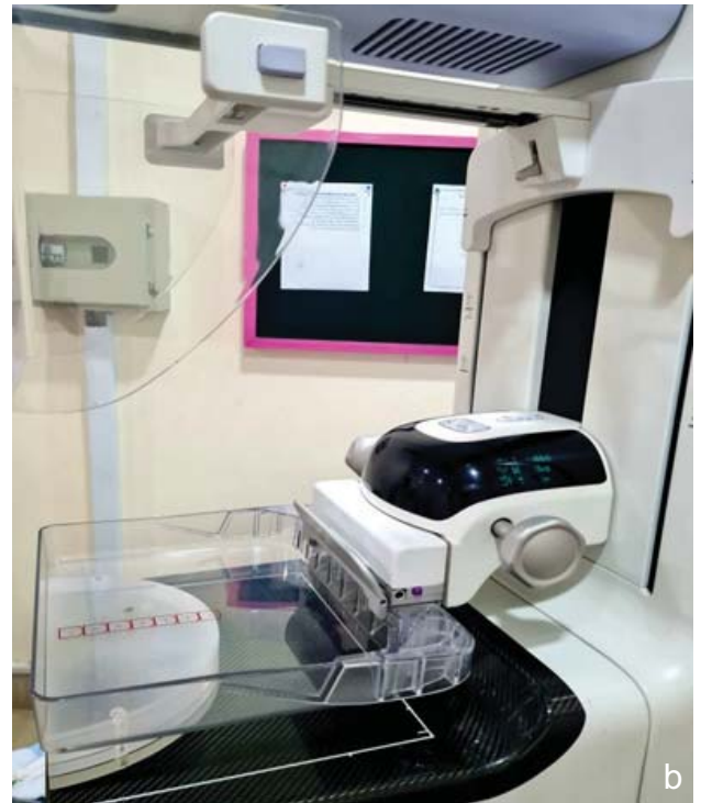
Figure 2: a) Air Kerma (K air ) setup of ACR Phantom, b) AEC measurement with PMMA Phantom
