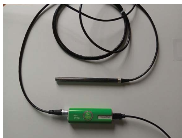
Figure 1: A calibrated ionization chamber (IC) (black) and a Magic Max basic unit (in green) for absorbance and transmission factor measurements
