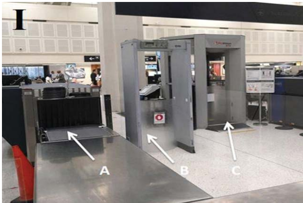
Figure 1: Airport machines from left to right (A) x-ray machine for luggage, (B) metal detector, and (C) MMW scanner for travelers.
